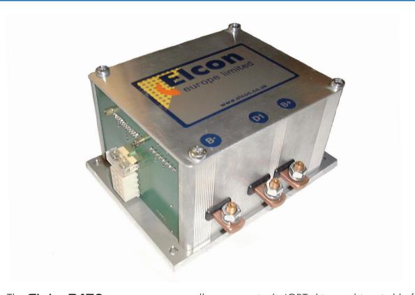
The **Simtec P450** pump motor controller, uses a single IGBT drive and is suitable for series wound motors.
